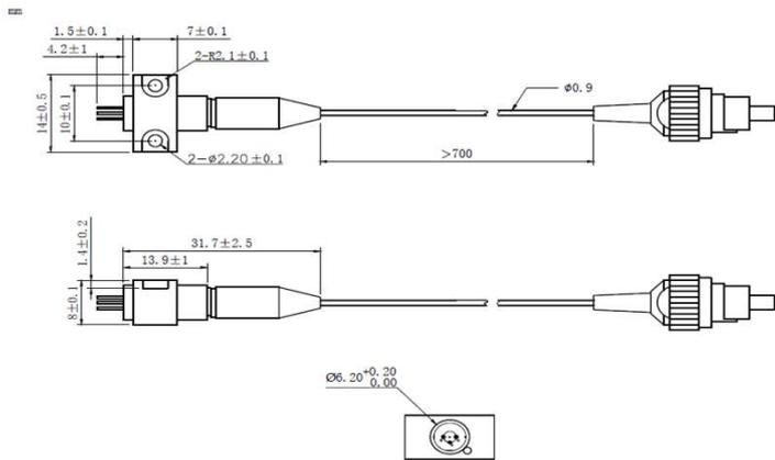
**Pin Bottom View (Coaxial, B82 Package) :**
